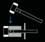
Tap the clamping pin into the bore hole.
