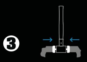
In the vice, press the new insert into the housing and insert retaining pins.
