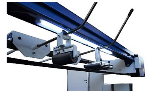
LIGHT POINT ON THE PLANE The light point on the worktop guarantees a better quality of work and facilitates the operator.
