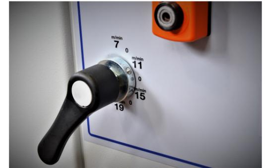
**FOUR FEED SPEED OF THICKNESS ROLLERS**
